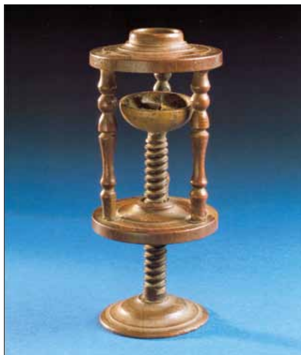
Fig. 1 Augsburg-type Screw-focus Simple Microscope.
